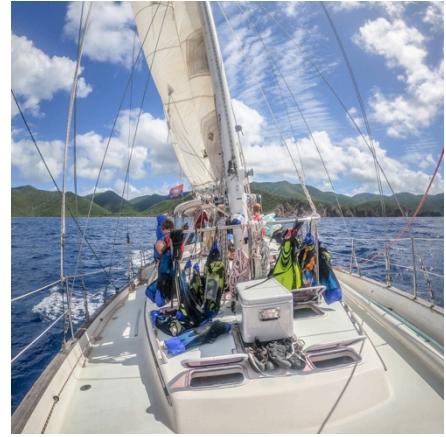
This shows the boat heeling, or leaning, due to the wind on the sails
