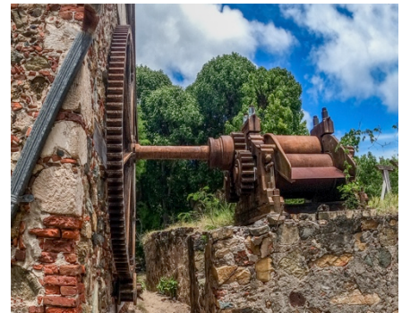
The power was then transferred to the rollers to crush the cane to yield juice
