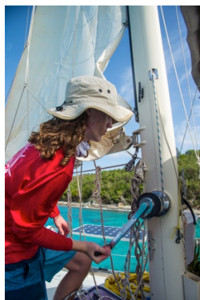
Once raised, the winch is used to tighten the sail
