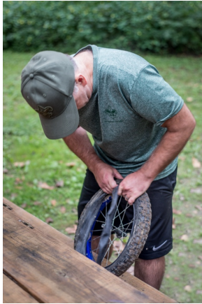
Mr. McGrath explaining how to replace an inner tube
